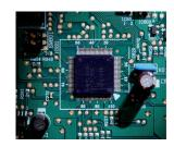
The vector-controlled inverter quickly converts current into a smooth sine curve to achieve smoother operation of the compressor's DC motor.
