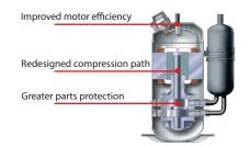
Optimization of discharge port positioning and blade thickness reduces the compression loss and friction resistance. Increasing the surface area of the rotor magnets and the addition of slits realize greater efficiency and reduced noise.
