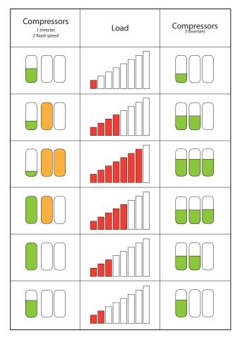
The graph shows how is effective the SMMS-i compared to other VRF systems. It is important to note that while at full capacity load the efficiency is similar (when the EER and COP are measured) and how effective is at lower capacities, resulting effective even down to 30%: a condition in which other systems cannot operate.
