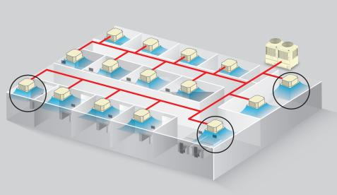
Refrigerant flow is adjusted to maintain consistent individual temperature control
