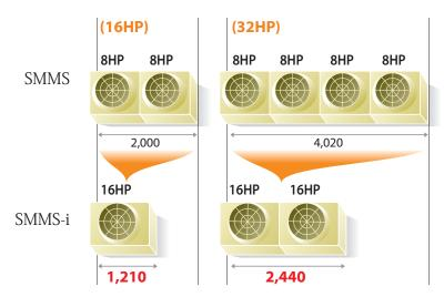
A 16HP system installation now occupies only 2/3 the footprint and weight of two units previously required.
