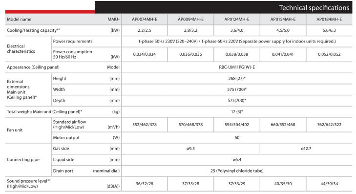
Figures in parentheses are for ceiling panels. This reference piping consists of 5 m of main piping and 2.5 m of branch piping connected at the same height level.
