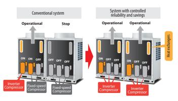
Using greater heat exchanger volume is more efficient 12
