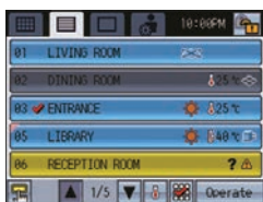
LIST screen Displays the detailed operation status of each group with group name.
