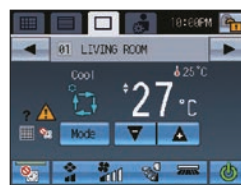
GROUP screen Displays the detailed operation status of each group. Sets group operations.
